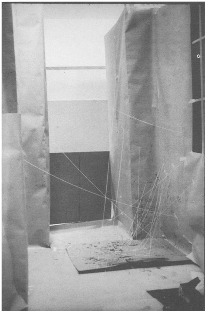
FIG. 6a—Illustration of the use of strings at the mock scene to determine the approximate point of origin selected blood spatters.
